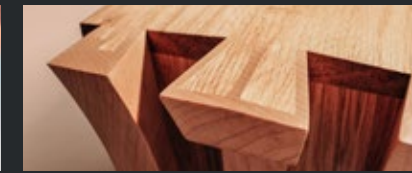
Half Lapped Dovetail
